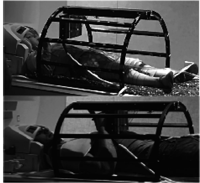
FIGURE 1 Experimental setup. Adults and children used the same apparatus and special care was taken to ensure the comfort of the participants. The MRItab, arm pillow, and Wheaton® elastic shoulder immobilizer were adjusted for each participant. Subject-specific adjustments ensured that the participants were in a comfortable writing position and could see the screen of the MRItab
